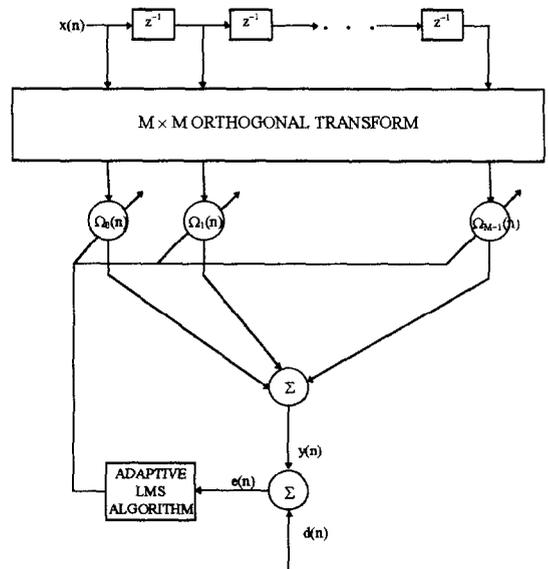
Figure 1 Block diagram of the Transform domain ADF
