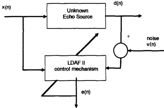
Figure 3 Block diagram of the LDAF II in echo cancellation
