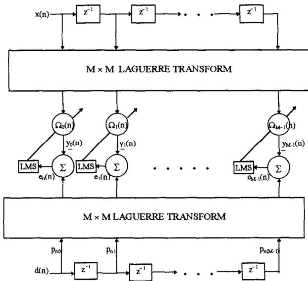
Figure 2 Block diagram of the Laguerre domain ADF
