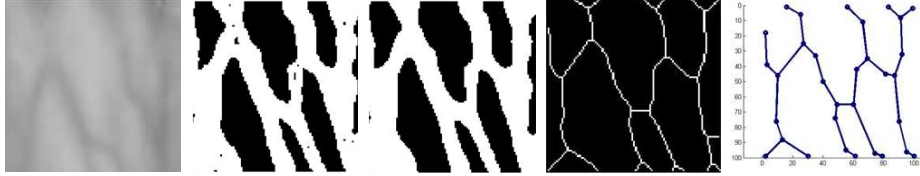
Fig. 6. LEM extraction steps: (left-to-right) A vein image, Yasuda binarization, noise removal, skeletonization and line segments generation
