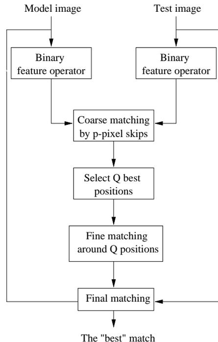
Figure 1: Three stage coarse-to-fine-final matching with recourse to original image pair.
