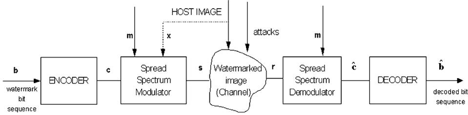
Fig. 1. Watermarking as a communications system.
