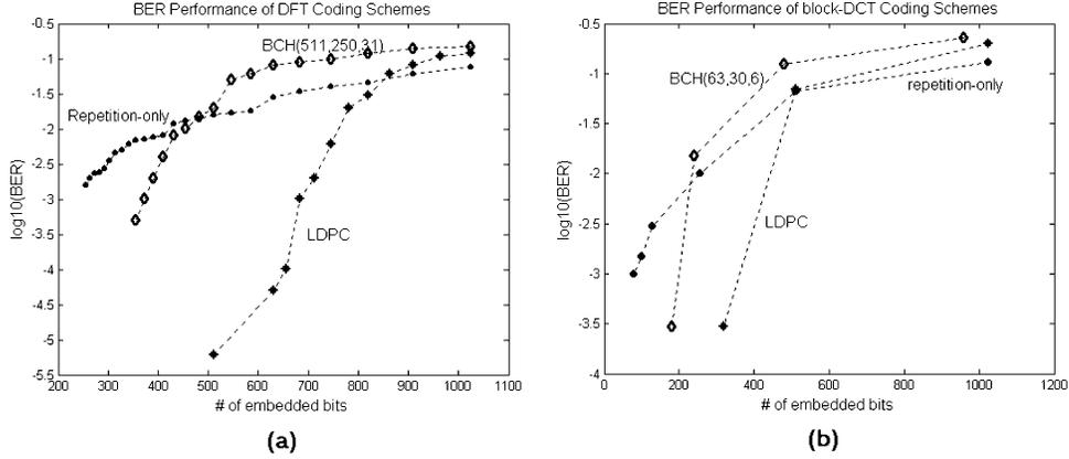
Fig. 2. BER performance of LDPC codes as compared to repetition and BCH codes. (a) DFT channel. (b) DCT channel.
